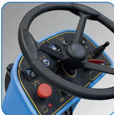
A 24 scrubbers are easy to use thanks to the simple and user friendly controls. From the control panel the operator can adjust the maximum forward speed and the quantity of cleaning solution outflow, selecting the options most suitable to the dirt type. Job is simplified and made faster by the automatic lifting of the squeegee and of the brush plate.
